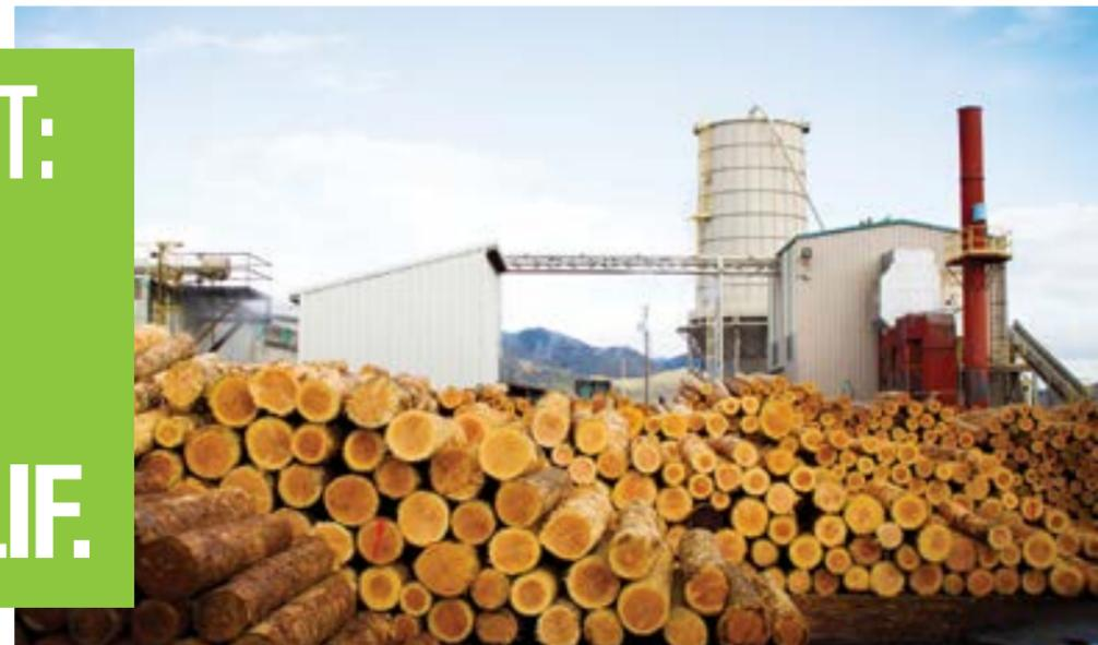
Some of the chips are used as fuel for Yreka's boiler. The machine generates the steam used to heat logs prior to peeling. Most of the chips are sent to other facilities to be turned into particle board, MDF (medium density fiberboard), paper pulp, and even electricity. "Burning the wood chips generates steam, which turns turbines that generate electricity," explained Don.
